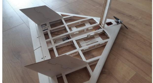
Front of rudder has both sides balsa strip precut
