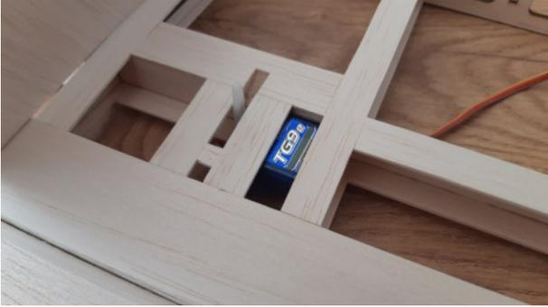
Servo comes locked partly in the spar and glued
